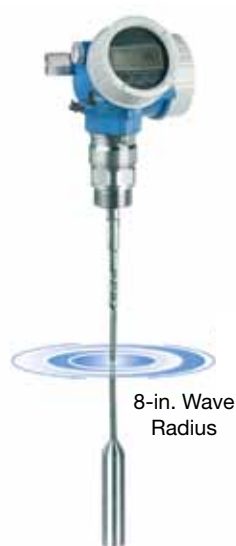
◀ Figure 3. In a guided-wave sensor, 80% of the emitted radar energy stays within an 8-in. radius of the wave guide, which provides increased accuracy.
